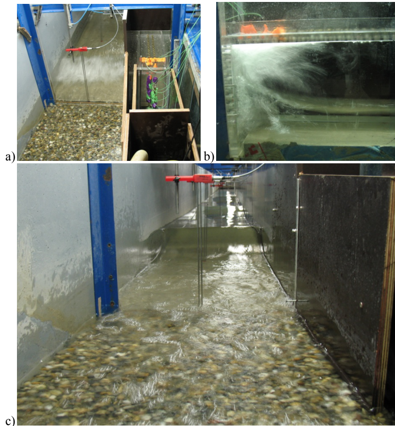
Figure 3.22. Top view of open end section, b) Side view closed end with scaled model c) Shows the guide wall along the flume
