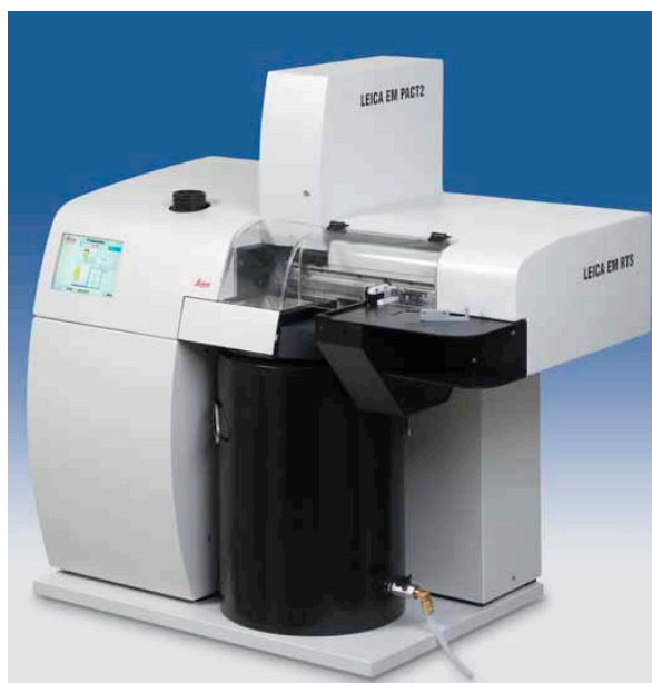
Figure 3.5: Leica EM PACT 2. Reproduced from Leica microsystems (2009).
