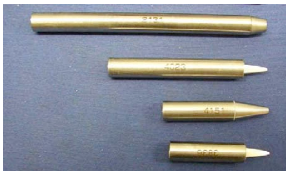
Figure 5.4: Different types of XOS polycapillary half-lenses which are available at beamline L. From top to bottom: conventional polycapillary, strongly-focusing polycapillary, high-energy polycapillary, detector polycapillary. The conventional polycapillary is 100 mm long. Reproduced from Falkenberg (2007a).
