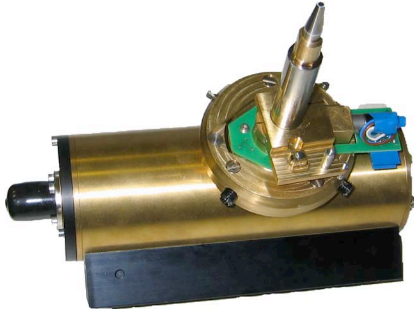
Figure 4.4: Rhodium X-Ray tube with attached polycapillary.
