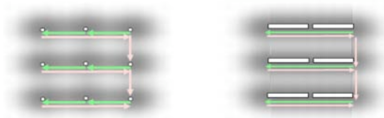
Figure 5.6: Principle of conventional (left) and continuous (right) scanning mode for 2-dimensional arrays of MCA spectra. Reproduced from Falkenberg et al. (2005).
