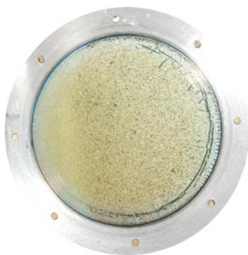
Figure 6.8: Prototype Free Standing Thin Film (FSTF).
