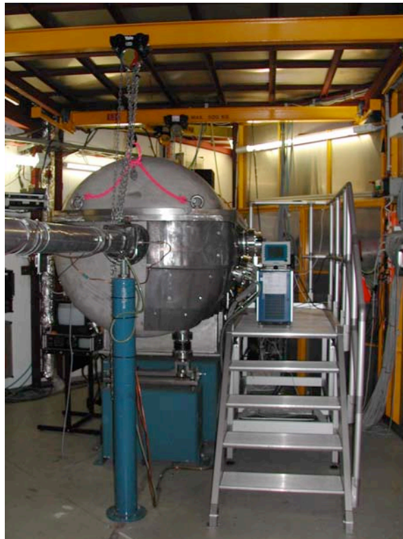
Figure 5.3: View of the operational monochromator. The shielded horizontal tube exiting the monochromator is the He -flushed X-ray beam-pipe, which extends towards the experimental table.
