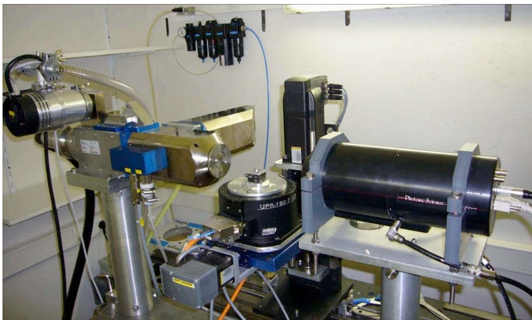
Figure 5.54: Absorption Tomography set-up at UGent.
