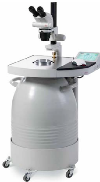
Figure 3.7: Leica EM AFS2. Reproduced from Leica microsystems (2009).
