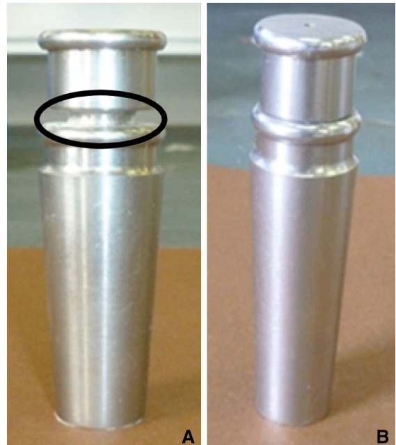
Fig. 3 A Plunger not in contact with the top of the container (cylinder inside diameter 12.70 \pm 0.10 mm) when blast furnace slag is measured, B perfect contact plunger with—top of container
