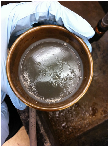
Fig. 2 BFS1 retained on no. 325 (45 \mu m) sieve after wet-sieving following ASTM C 430
