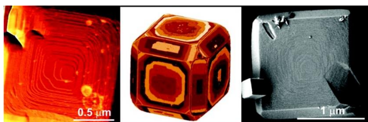
Figure 3.2.3: AFM image, Monte Carlo solution and HRSEM image for Zeolite A in medium supersaturation conditions. Reprinted with permission of ref. 69 .
