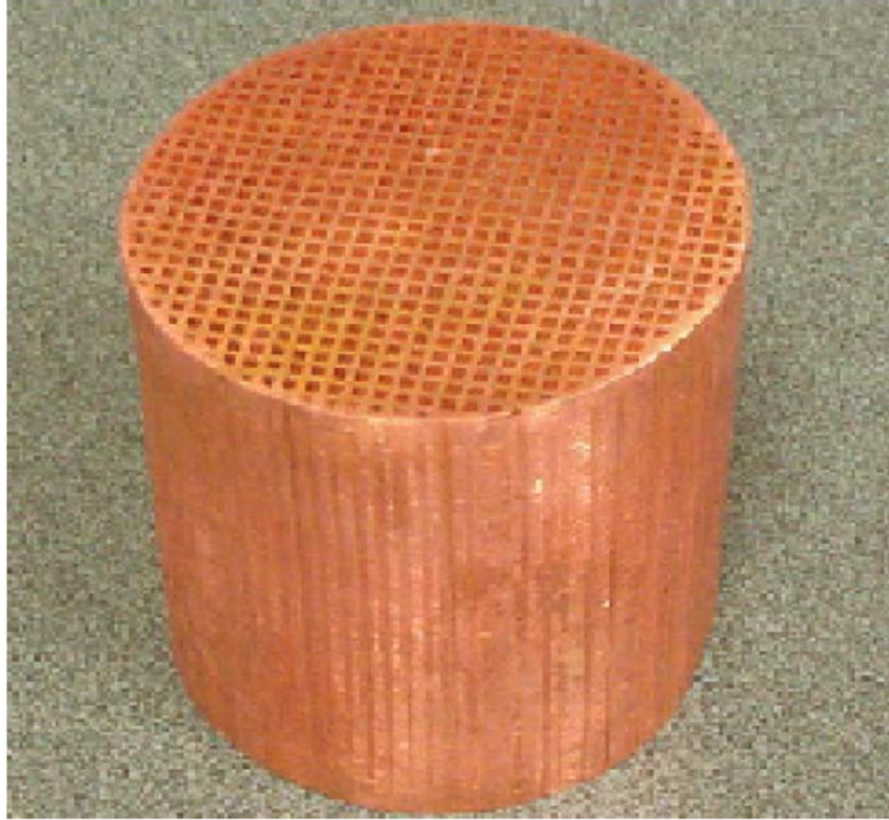
Fig. 9. Copper based monolith catalyst support: a square celled LCA, Boger and Heibel [67].
