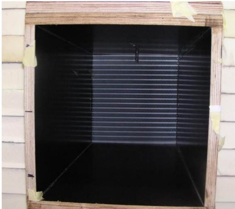
Figure 5 Illustration of the insulated part of the test rig
