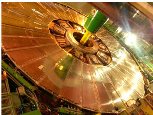
Figure 6. One of the two CMS endcap disks fully instrumented with RPC detectors.
