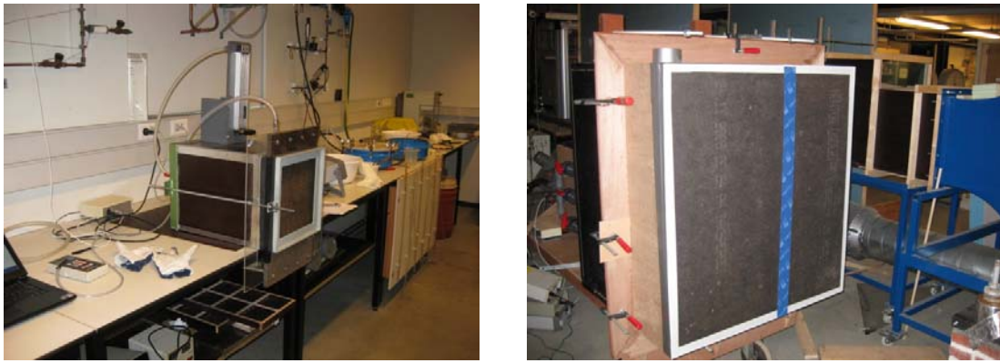
Figure 6 Laboratory test equipment to determine air permeability on material and assembly level.
