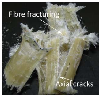
(a) Final deformation patterns (top - HXST1; bottom - HXDT2).
