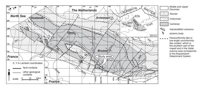
**Figure 1 :** Geological subcrop map of the Brabant Massif, after De Vos et al. (1993) and Van Grootel et al. (1997), with location of the study area (see also Fig. 2) and position of the Brabant Massif within Avalonia, as the southeastern part of the Anglo-Brabant Deformation Belt (ABDB), flanking the Midlands Microcraton (MM) (upper right inset).
