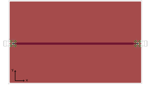
Fig. 13. Device under test : straight microstrip
