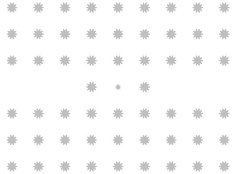
Fig. 16. EC filter with starlike dielectric cylinders.
