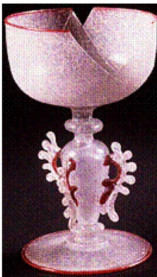
Fig. 5. Severely crizzled 17th or 18th century Venetian white glass goblet (Courtesy: V.L. Oakley, V & A collection of glasses and ceramics).
