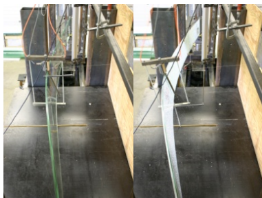
Fig. 4 - Buckled beam before and after the breakage of one sheet
