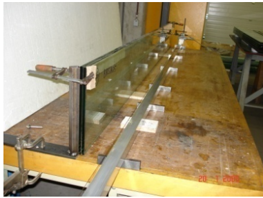
Fig. 1 - Continuous measurement of the shape imperfections
