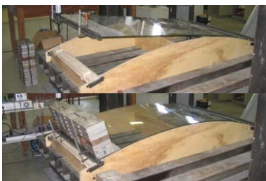
Fig. 11 - Cold bending of laminated hardened glass.
