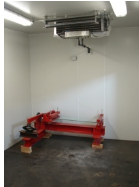
Fig 9 - Torsion test set-up in climate-controlled chamber
