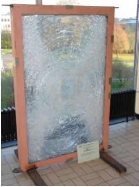
Fig. 13 - Broken prison glazing after static loading test
