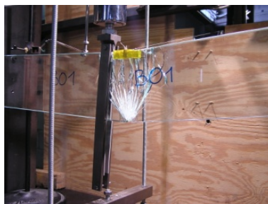
Fig. 5 - Broken laminated, annealed floatglas
