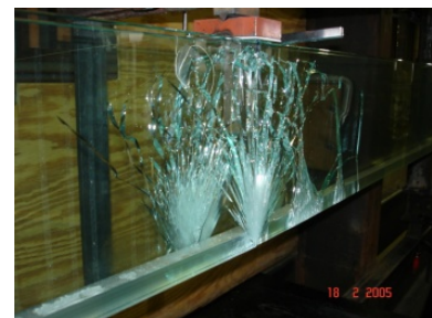
Fig. 6 - Broken reinforced laminated, annealed floatglas
