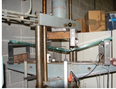
Fig. 8 - Destructive four-point bending test on a laminated glass plate
