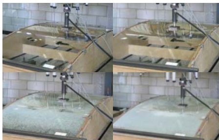
Fig. 12 - Unloaded, loaded, one ply broken, both plies broken.
