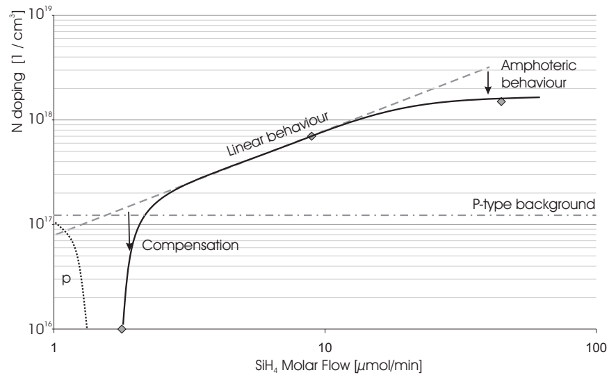
Figure 4-16 N-type doping behaviour of Al_{35}Ga_{65}As using silane and TBAs
