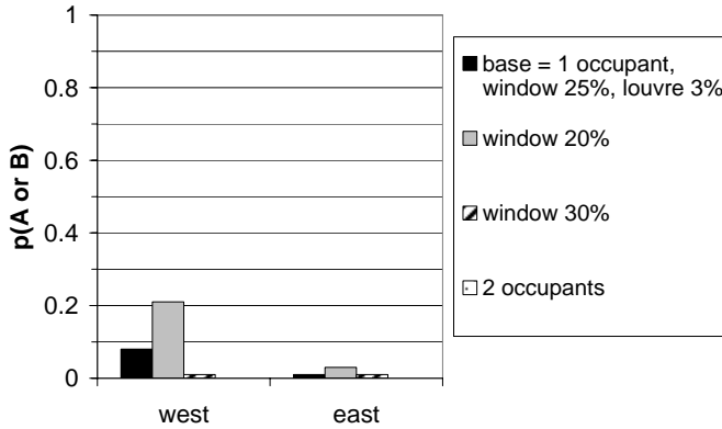
Fig. 5.40 Comparison of the impact of window area and occupancy on the uncertainty of thermal comfort based on ATG
