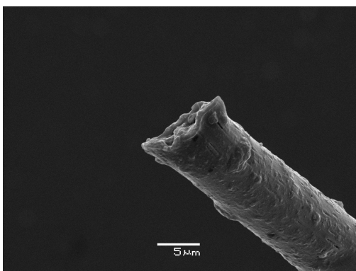
Figure 10.21 - SEM photo of fracture surface (broken at 20 mm/min)
