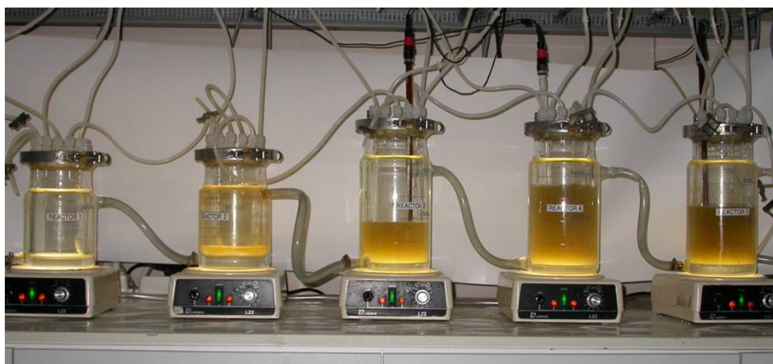
Figure 3.1 Picture of the Simulator of the Human Intestinal Microbial Ecosystem (SHIME). Vessels 1 to 5 respectively simulate conditions from the stomach, small intestine, colon ascendens, colon transversum and colon descendens.
