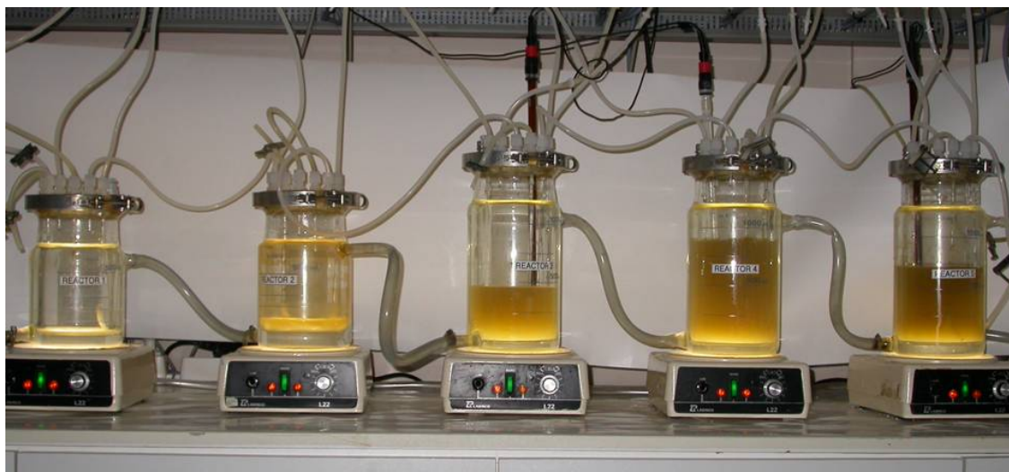
Figure 1.15 Laboratory setup of the Simulator of the Human Intestinal Microbial Ecosystem at LabMET.
