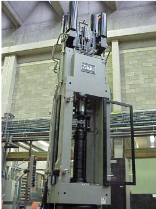
Figure 5.1 MTS compression machine
