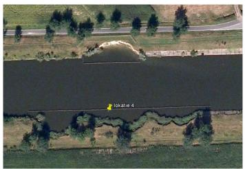
Figure B.1: Plan view of the monitored location 4, which consists of a single row of off-bank timber piling, parallel to the fairway and without bank connection. A reed belt additionally protects the eroded river bank. At the opposed bank side, a layout of this nature-friendly bank protection with bank-connected timber piling and without reed belt is shown. (source: Google Earth)
