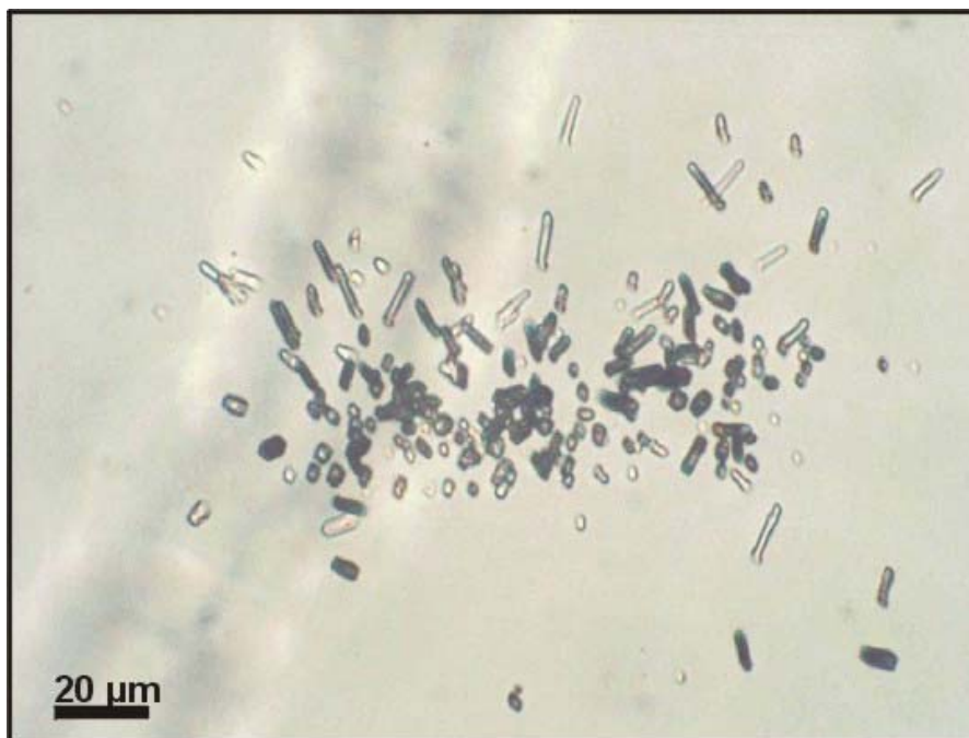
Figure 1.11: Fission tracks in a muscovite ED after etching in 40% HF for 30 minutes at 25°C.
