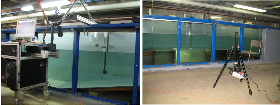
Figure VII-7: Set-up for capturing the flow field around the base of the vertical pile in the large wave flume: under water light sheet optics (left) and camera position, pile and mirror (right)
