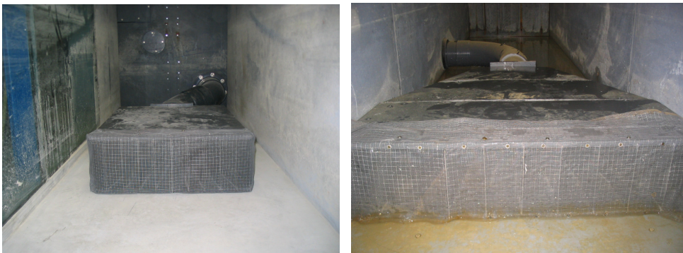
Figure II.6: Picture of the pump in- and outlet in the flume
