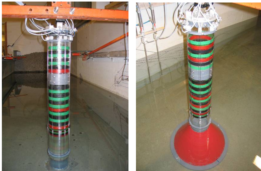
Figure 6-4: Mounted capacitance wave gauges on monopile and cone foundation.
