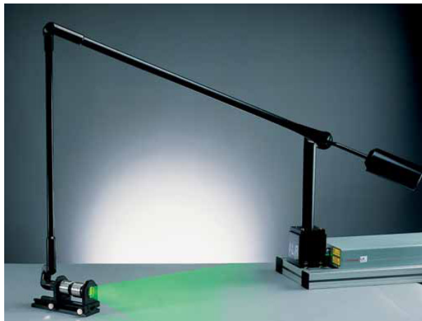
Figure VII-2: Laser arm, light sheet optic of the PIV system
