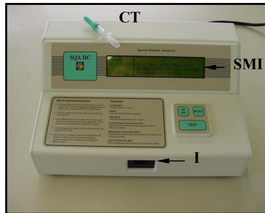
Figure 1. Sperm Quality Analyzer (SQA): the capillary tube (CT) is filled with the semen sample and inserted (I) in the SQA; after 45 seconds the Sperm Motility Index (SMI) is displayed taking into account the motility, the morphology and the concentration of the semen sample.
