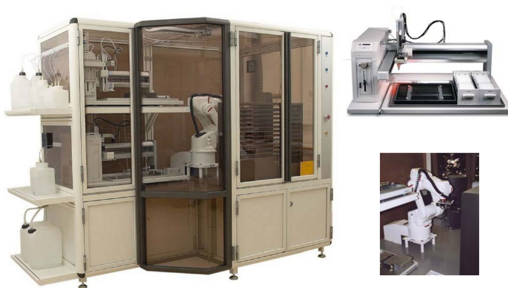
Figure 3.30. The Ettan™ Spot Handling Workstation from GE Healthcare (CRPGL, Luxembourg). Spot picking, destaining, trypsin digestion, peptide extraction and sample spotting for MALDI MS analysis are integrated. The blow-ups show the spot picker and the robotic arm that transports the samples between the different modules.
