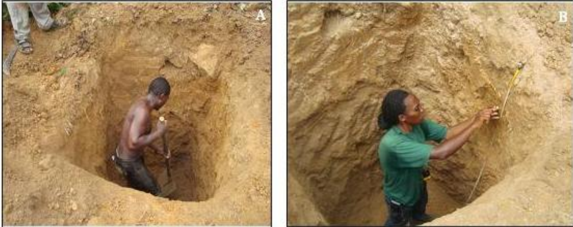
Fig. 3. 2. View of geometric configuration of Pit 1 dug into a slides scar at Bonjo: a) digging pits; b) in situ measurement of relative shear strength with a Torvane meter.
