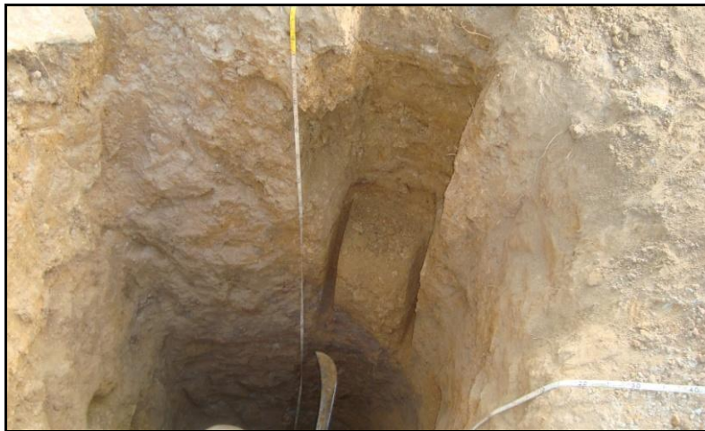
Fig. 3. 3. Collecting block samples for laboratory analysis from the wall of a pit sunk at Bonjo. Note sharp the colour transition on the walls of the pit.
