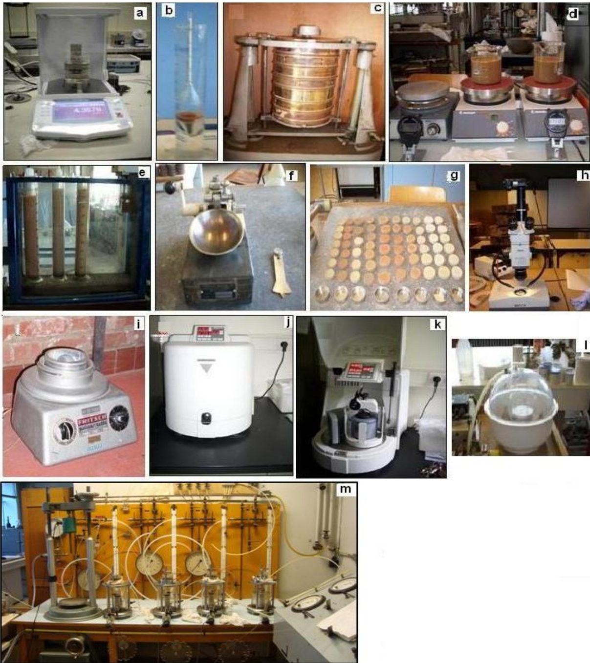
Fig. 3. 4. Catalogue of the laboratory equipment used for sample analysis: a) electronic balance used to determine sample bulk density; b) hydrometer; c) sieves and mechanical sieve shaker used for separating particles into different fractions; d) magnetic stirrer; e) 1 litre sample solution in a water bath for measuring the silt and clay fractions within each sample through sedimentometry; f) Casagrande apparatus used in the determination of liquid limits; g) shrinkage dish for linear shrinkage measurements; h) petrologic microscope; i) agate ball mill; j) external view; k) internal view of agate ball mill used for the preparation of sample powders for ICP-OES analysis; l) pressure chamber with pycnometer used for the determination of the specific gravity of the solid particles; m) three automated triaxial cells.
