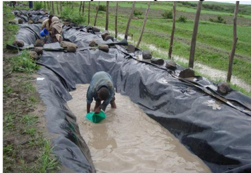
Fig. 3. Partial view of the experimental plot at Adi Gudom. On a daily base in the rainy season, and after measurements and samples are taken, the collector trenches are emptied. The runoff plots are located at left.
