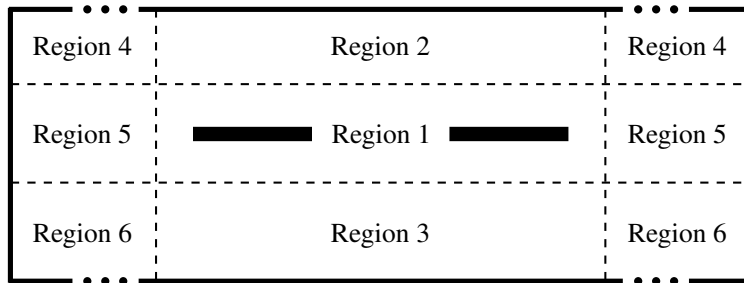
Figure 11. Subgridding regions to discretize the differential stripline pair
