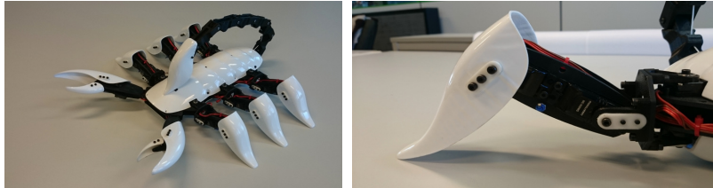
Figure 4. Finished scorpion hexapod robot (left) and detail picture of the leg design (right)
