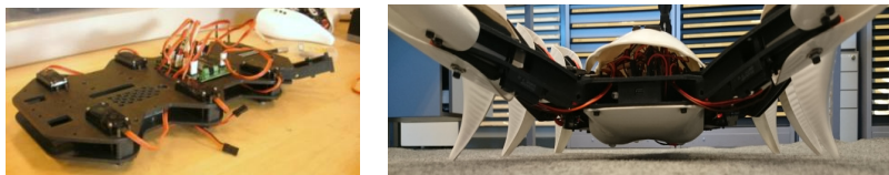
Figure 10. Final scorpion body, existing of two laser cut ABS- plates and thermoformed PS shells
