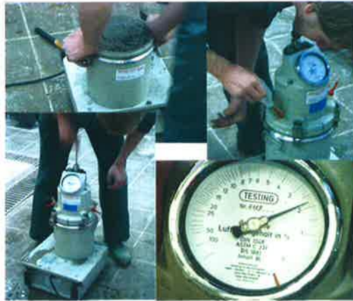
Figure 1 – Determination of air content in accordance with NBN EN 12350-7
