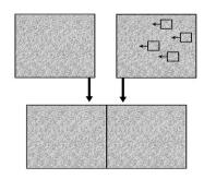
Fig. 1. Stereograms in active stereogram test. In this example, 4 squares are cut out and moved horizontally.
