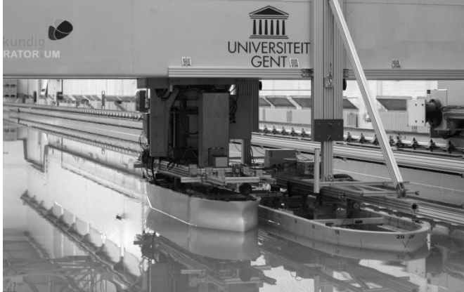
Fig. 1. Both ship models attached to the main carriage of the towing tank.
