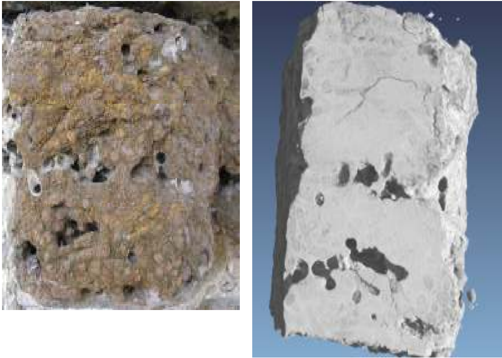
Figure 8: Bioturbated ferruginous sandstone (length: 14 cm ; width: 10 cm) heavily attacked by mason bees (recent perforations marked by light grey clay lining), extracted from the Maagdentoren (left). The corresponding CT-scan (right) shows the original burrows by sea organisms (worm-like faint grey bioturbations), most clearly visible in the upper part of the scan, and similar zones which attracted the mason bees whose perforations are visible in the middle and the lower part of the scan.
