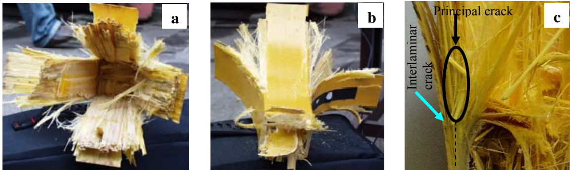
Figure 7 (a & b): Failure pattern of SP1 series (c) Cut section of the tube
