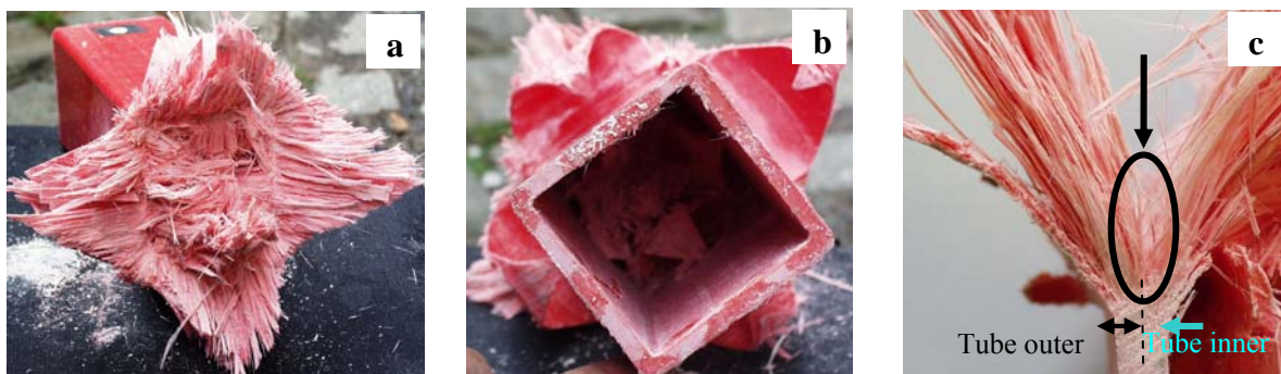
Figure 8 (a & b): Failure pattern of SP2 series (c) Cut section of the tube
