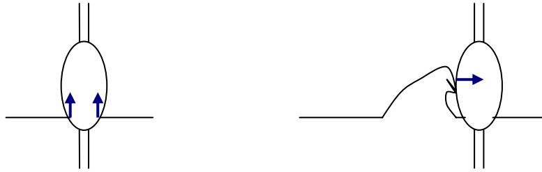
Figure 5: Egg bottom slamming (left) and egg breaking wave slamming (right)
