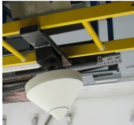
Figure 8: cone test sample attached to the ladder
