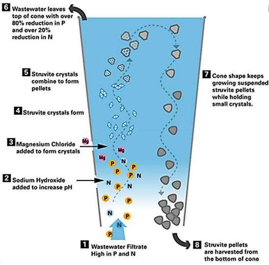
Design: Fluidized bed reactor or continuously stirred tank reactor
