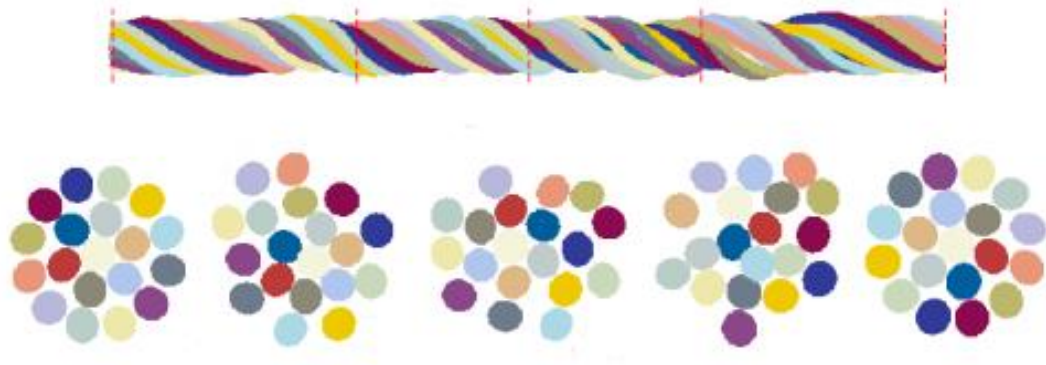
Figure 1: The twisting of a textile yarn simulated by discretizing the yarn into 19 virtual fibres and applying twist on the yarn ends shows that the modelling method captures the fibrous behaviour in a natural manner.
