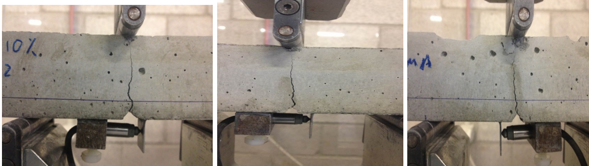
Figure 1: Mortar samples containing one capsule from PLA+10% impact modifier (left), PLA (middle) and PMMA (right) after three-point-bending test (crack width:0.9 mm)
