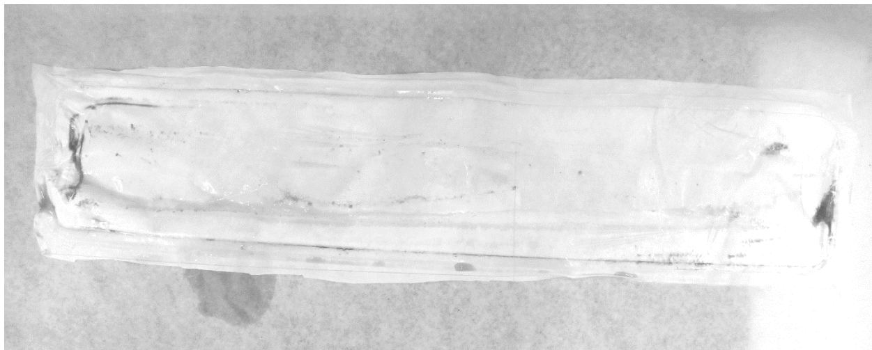
Figure 9: Membrane fouling of the membrane used in experiment of Figure 10.
