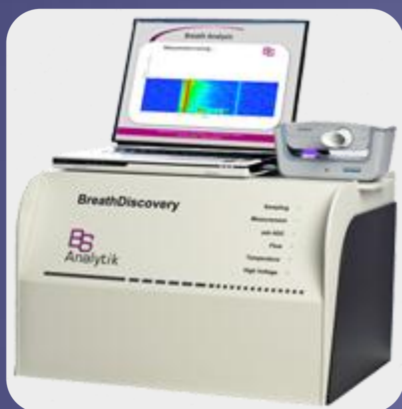
Figure 2: The MCC/IMS device (BioScout) with sampling unit (SpiroScout).
