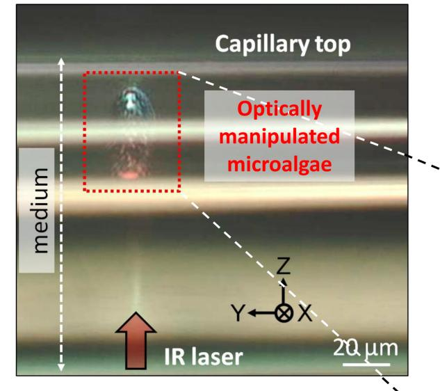
Optically levitated S. trochoidea microalgae in aqueous medium, translated to the upper capillary wall to prevent X-ray induced vertical sample movement during a progressing scan [3].
