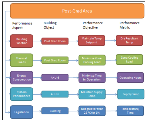
Figure 4: Scenario Modelling Framework, illustrating performance assessment criteria for an office space
