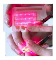
Left : Ultra-thin chip package; right : 15-LED stretchable circuit, before (top) and during (bottom) extreme deformation
