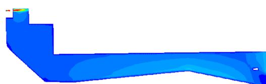
Figure 4. Comparison between velocity profiles at different depths from bottom of the F1 pond (scenario 2005).
