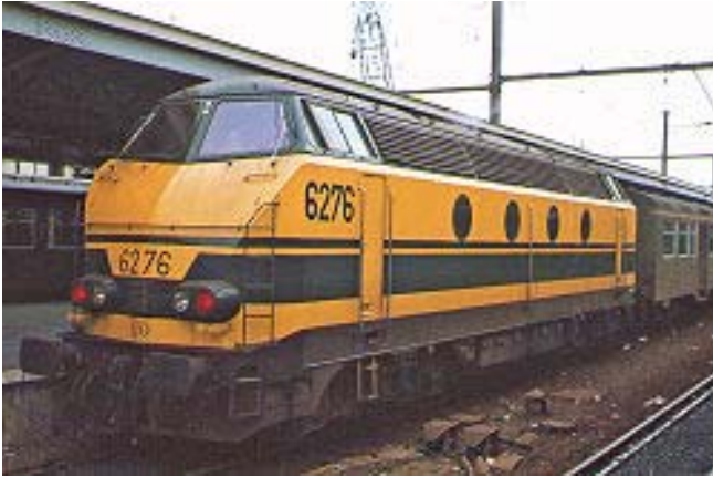
Fig 7 Diesel-electric locomotive 1961, using DC machines (La Brugeoise & Nivelles) [4]
