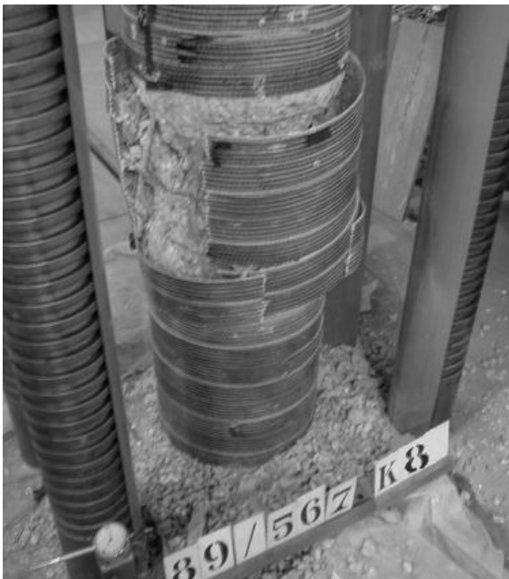
Figure 1a. Failure of HFRP fully wrapped column.
