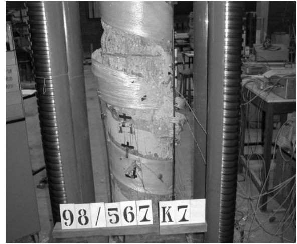
Figure 1b. Failure of GFRP partially wrapped column.
