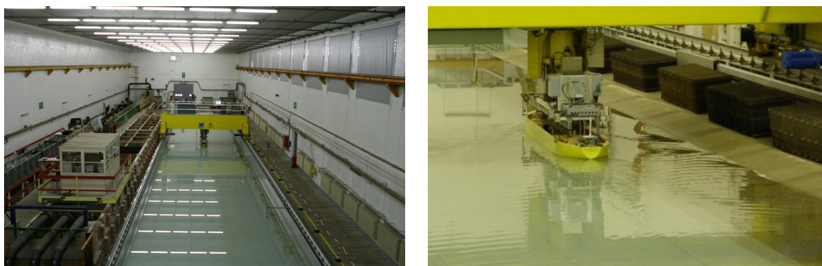
Figure 3: 8,000 TEU ship model tested in the Towing Tank for Manoeuvres in Shallow Water
