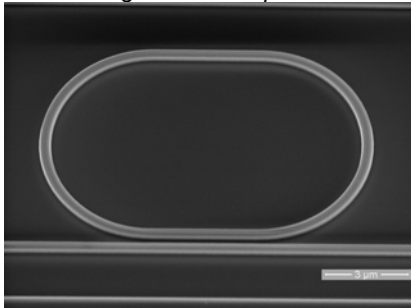
Figure 3. Race track ring resonator
