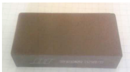
Fig. 20b. Iron powder yokes 60x30x15 mm bricks (Magnetics Spang)
