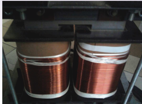
Detail of a glued coil formers, large UU inductor with iron core, adjustable air gap
