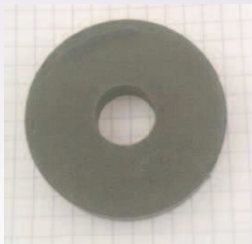
Fig. 20a. Ferrite disc with hole 50/15/10, low frequency high induction ferrite (unknown brand)
