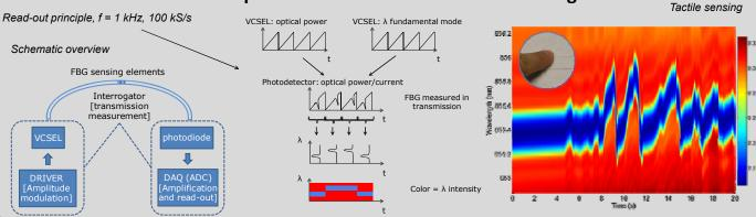
**Conclusion** We have developed an integrated fiber sensing system including embedded fiber sensors and low-cost compact fiber coupled driving and read-out optoelectronics. Dynamic interrogation of fiber Bragg gratings is demonstrated enabling high accurate and robust sensing in harsh environments.
