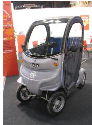
Fig. 8: electric covered light vehicle (Ducati Free Dug, 240kg) [8]
